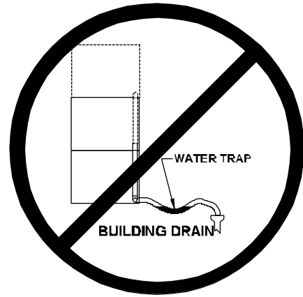
IMPROPER DRAIN LINE CONNECTION
