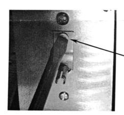
Install the spring over thermostat shaft as shown (arrow). Install the counter-sink screw included with the spring. Tighten the screw, ensuring the spring is positioned as illustrated (arrow).
