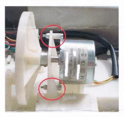
Ensure that the centre of the shaft is in the centre of the support bracket hole so that the CAM wheel activates the microswitch correctly.
