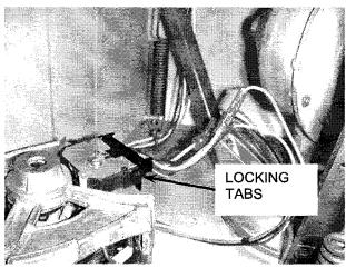
Connect the connector of the harness to the motor.
