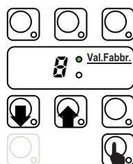
Fig. 23 Change time activation (Tank LED indicates default)
