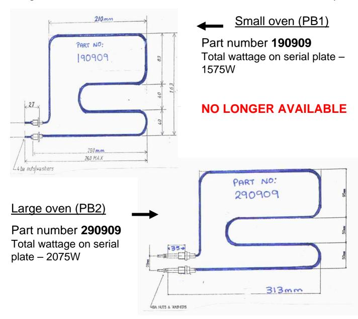
Main oven elements for non-fan assisted small Potato Bakers (PB1models)
