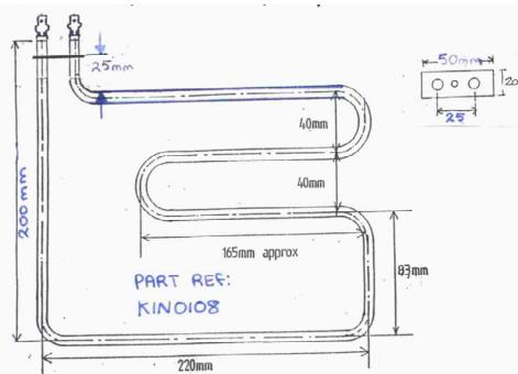
Main oven elements for non-fan assisted large Potato Bakers (PB2 models)
