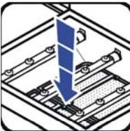
*Check whether drainage filter, pump suction filter and surface strainers are installed.*
