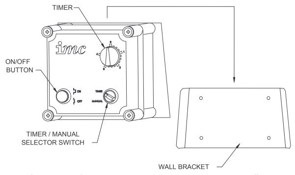
Note: Control boxes for three phase machines have separate on and off buttons.
